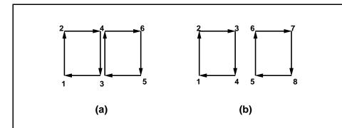
Figure 2.5. (a) A quad strip. (b) Independent quads. The numbers give the sequencing of the vertices between **Begin** and **End**.
