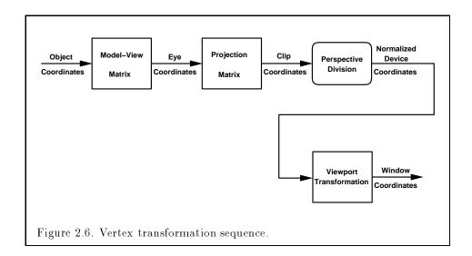
If a vertex in object coordinates is given by  $\begin{pmatrix} x_o \\ y_o \\ z_o \\ w_o \end{pmatrix}$  and the model-view
