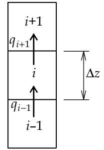
$$\frac{h_{i-1} - 2h_i + h_{i+1}}{\Delta z^2} = \frac{S_s}{k} \cdot \frac{\partial h_i}{\partial t}$$
