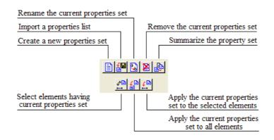
To create a new set of properties, select the button 🗈 and assign the new set a unique name. The button 🖾 imports a list of property sets from another file generated by FTOOL. Duplicate property sets in the imported file are ignored. The internal function
