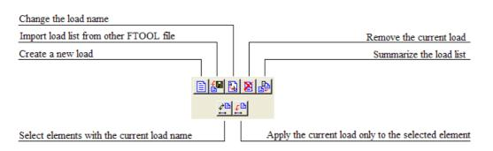
The icons shown in the figure below are used to manipulate the load in a list:
