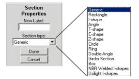
Based on the type of section selected, the parameters that define the features of that section are then defined along the side of the screen under the schematic drawing.
