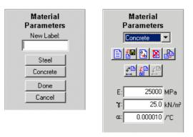
Material parameters include Young's modulus, specific weight (not currently used by FTOOL) and coefficient of thermal expansion (if temperature loadings are applied).
