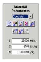
Material parameters include Young's modulus, specific weight (not currently used by FTOOL) and coefficient of thermal expansion (if temperature loadings are applied).
