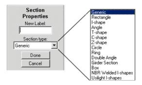
Based on the type of section selected, the parameters that define the features of that section are then defined along the side of the screen under the schematic drawing.
