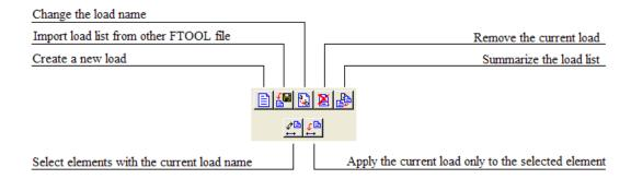
The current load will be applied to the selected elements (members or nodes). The members of interest must be selected and the load is applied through the button for members, or the button for the nodes.
