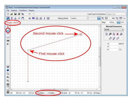
Member and node creation is straightforward. To insert a member, select the button  $\square$  and click on two points within the model display area. Nodes are created instantly at the ends of the member. If
