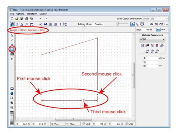
*Dimension Lines* are auxiliary lines used to indicate distances on the structural model. To insert a dimension line, select the button in the Edit toolbar and click three points on the screen. The two first points are the control points to specify the distance to be listed by the dimension. The third point defines where the dimension line will be located. During the construction of the line, the program updates the dimension line on the screen until the user enters the third point.
